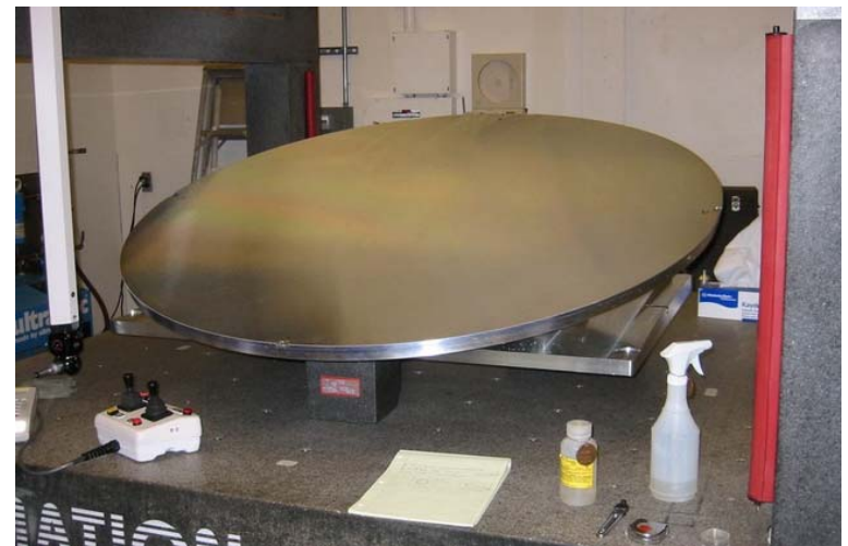
1.5 m diameter tertiary mirror
